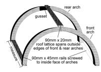
Unlike the rails, each roof lattice piece is screwed on top of the front and back arches, not between them. so take an overall measurement of the left rail and front and rear arch
