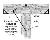
Measure from the very top of the "T" crossbar to 762mm down the trunk of the "T." At this point (and centred from side to side), drive in a nail and tie a long (non stretchy) string to it. At the string's opposite end, tie a pencil so that, when the string is taut, the pencil is 762mm from the nail. Now, you have a reliable tool for drawing the arches. Alternatively you could use a narrow strip of ply with a nail in
