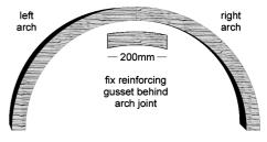
Follow the tracing with your jigsaw and cut out the gusset. Then cut out a second gusset, so there's one for both front and back arches.
