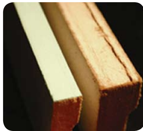
ULTRAprime™ and an alternative product were subjected to a 24 hour water submersion test. Unlike the alternative product tested, ULTRAprime™ (left) did not show evidence of cracks or splits.
